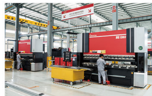
日本天田九轴数控折弯机 Japan AMADA nine-axis CNC bending machine
