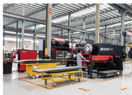
日本天田多工位转塔冲床 Japan AMADA multi-station turret punch press
