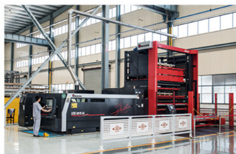
日本天田光纤激光切割机 Japan AMADA optical fiber laser cutting machine
